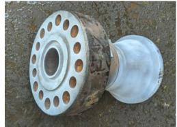
UNIT S/N: B3089830-1 INSPECTION RESULT: VISUAL & MAGNETIC PARTICLE INSPECTION (M.P.I.) HAD BEEN DONEON THE **VISUAL, THOROUGH EXAMINATION** AVAILABLE AREAS FOR THE ABOVE DESCRIPTION Avaliable critical areas inspected MAGNETIC PARTICLE INSPECTION and found free from cracks and other defects **FINAL RESULTS** THE ABOVE INSPECTED AREAS WAS ACCEPTED
