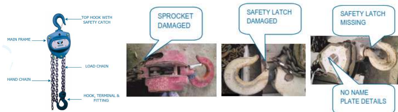
FIGURE (2): Inspection points and possible defects of hand operated chain blocks.
