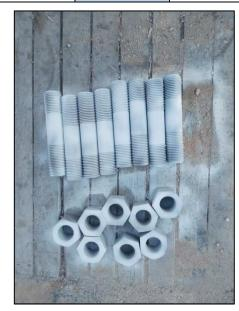
**NDT Equipment Details** Standard ASTM E709 Viewing Condition: Colored Media Method WET Yoke Permanent Serial No: PY-09 Due Date 15-08-2024 White Contrast WCP-2 Batch No: 220602 06-2025 Due Date Black Ink 7HF Batch No: 220605 Due Date 7-1-2025
