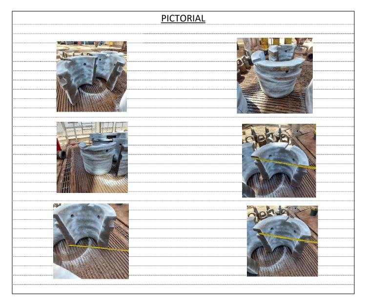
Remarks: CAT IV Inspection Was Carried Out on INSERT BUSHING BOWL and Found Accepted at The Time of Inspection.
