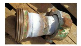
X-OVER 3" 206 WING X 4" 206 THREAD UNIT DESCRIPTION: UNIT S/N: TSS 307 INSPECTION RESULT: VISUAL & MAGNETIC PARTICLE INSPECTION (M.P.I.) HAD BEEN DONEON THE **VISUAL, THOROUGH EXAMINATION** AVAILABLE AREAS FOR THE ABOVE DESCRIPTION Thread & Avaliable critical areas inspected MAGNETIC PARTICLE INSPECTION and found free from cracks and other defects THE ABOVE INSPECTED AREAS WAS ACCEPTED **FINAL RESULTS**
