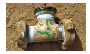
UNIT DESCRIPTION: TEE 4" 206 WING X THREAD X WING **TSS 318** UNIT S/N: INSPECTION RESULT: VISUAL & MAGNETIC PARTICLE INSPECTION (M.P.I.) HAD BEEN DONEON THE **VISUAL, THOROUGH EXAMINATION** AVAILABLE AREAS FOR THE ABOVE DESCRIPTION Thread & Avaliable critical areas inspected MAGNETIC PARTICLE INSPECTION and found free from cracks and other defects **FINAL RESULTS** THE ABOVE INSPECTED AREAS WAS ACCEPTED
