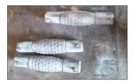
UNIT DESCRIPTION: ROLLER REAMER BLADE CUTTER UNIT S/N: CT-122B-D8048A,CT-122B-D8048B,CT-122B-D8048C **INSPECTION RESULT:** VISUAL & MAGNETIC PARTICLE INSPECTION (M.P.I.) HAD BEEN DONEON **VISUAL, THOROUGH EXAMINATION** THE AVAILABLE AREAS FOR THE ABOVE DESCRIPTION Avalibel Critical areas inspected MAGNETIC PARTICLE INSPECTION and found free from cracks and other defects unit found satisfactory and free of defects FINAL RESULTS at the time of inspection
