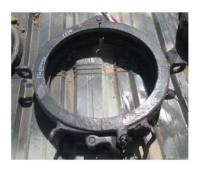
**UNIT DESCRIPTION:** SINGLE JOINTS ELEVATOR **BGGSJ002-18** UNIT S/N: **UNIT SIZE & SWL:** 5 Ton / 18 5/8" **INSPECTION RESULT:** VISUALLY INSPECTED AND FOUND FREE FROM DEFORMATIONS. VISUAL, THOROUGH EXAMINATION CORROSIONS, AND OTHER DEFECTS. M.P.I HAS BEEN DONE ON AVAILABLE CRITICAL AREAS AND FOUND MAGNETIC PARTICLE INSPECTION FREE FROM CRACKS AND OTHER DEFECTS THE ABOVE INSPECTED AREAS WAS ACCEPTED AT THE TIME OF FINAL RESULTS INSPECTION
