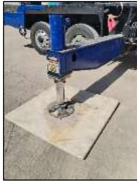
Crane front piston & Outriggers, found satisfactory at the time of inspection
