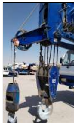
Main Block Hoisting & Whip line Hoisting, Boom With Radius Reading Limit Switches. All found satisfactory at the time of inspection
