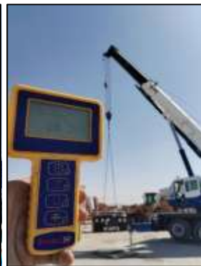
Crane Load Indicator & Radius 9 m , Boom Length 18.8 m, Load Chart SWL 14.3 Ton , Applied Load 14.2 Ton , As Per Load Chart, found satisfactory at the time of inspection
