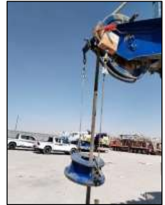
Main Hoist Block & Auxiliary Hoist Limit Switches Stopper All found satisfactory at the time of inspection
