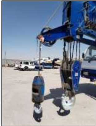
Main Hoist Block & Whip line Sheaves found satisfactory at the time of inspection
