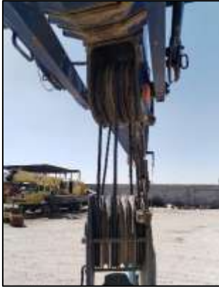
Main Hoist Block & Whip line Sheaves found satisfactory at the time of inspection
