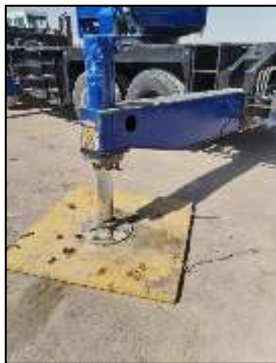
Crane front piston & Outriggers, found satisfactory at the time of inspection
