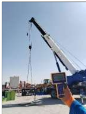
Crane Load Indicator & Radius 9 m , Boom Length 18.8 m, Load Chart SWL 14.3 Ton , Applied Load 14.2 Ton , As Per Load Chart, found satisfactory at the time of inspection
