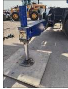
Crane front piston & Outriggers, found satisfactory at the time of inspection
