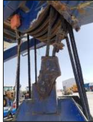
Crane wedge sockets & Wire Ropes Termination found satisfactory at the time of inspection
