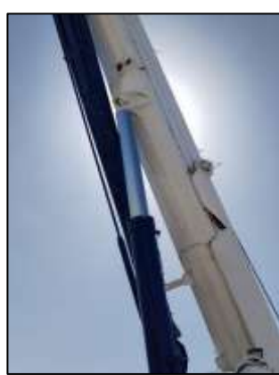
Boom Cylinder & Piping, Boom Sections, found satisfactory at the time of inspection
