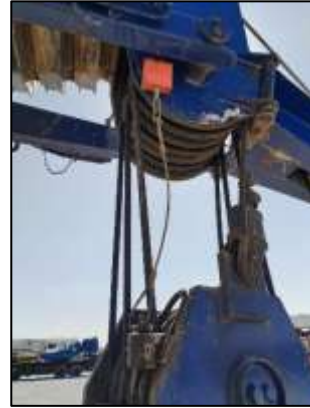
Main Hoist Block & Auxiliary Hoist Limit Switches Stopper All found satisfactory at the time of inspection
