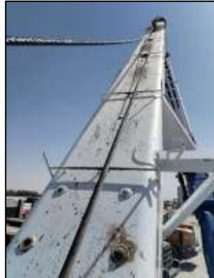
Wire ropes & Drum Reeving Functions, Rollers, Sheaves, found satisfactory at the time of inspection
