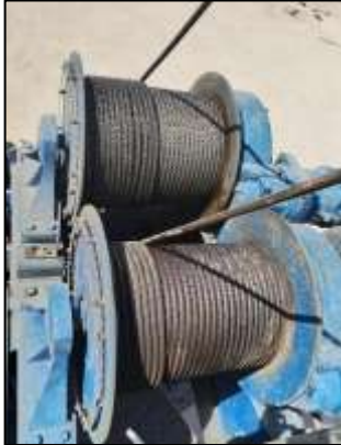
Wire ropes & Drum Reeving Functions, Rollers, Sheaves, found satisfactory at the time of inspection
